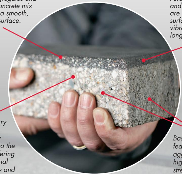
*Proprietary face-mix integrally bonded to the base, offering exceptional durability and aesthetic design.*
